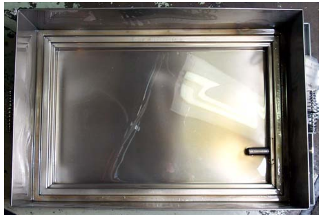
Filter pan with cover removed.
